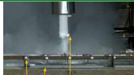
Thermocouples Substrate Release point Thermocouples and concentration sensor intakes
