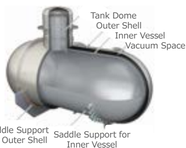
Vacuum Insulated Double Shell Structure
